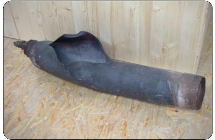
fig. 1 Exploded acetylene gas tank shown as a reminder of gas tank risks at a recent crafts exhibition at Munich. ©Spirig
