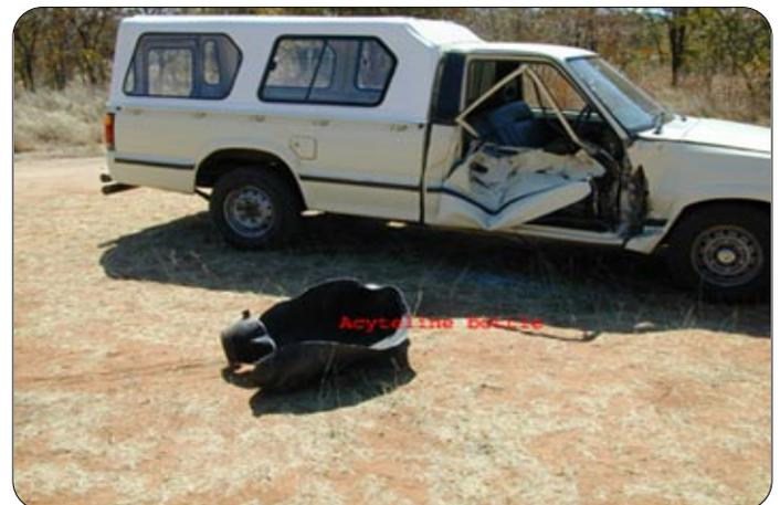
fig. 3 The exploded acetylene gas tank traveled almost 200 meters before hitting on a nearby parking lot the side of a car. ©Spirig
