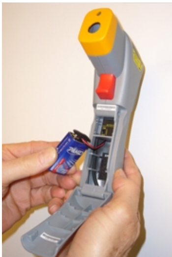
Install the 9-Volt battery. Select on / off for laser pointer, select °C / °F display in the battery compartment.
