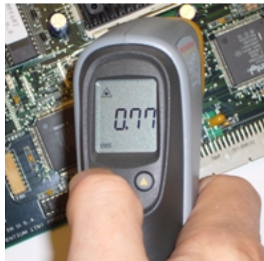
The CMI-056V has an adjustable E-Factor (0.10 to 1.00). The chosen value will be automatically saved.
